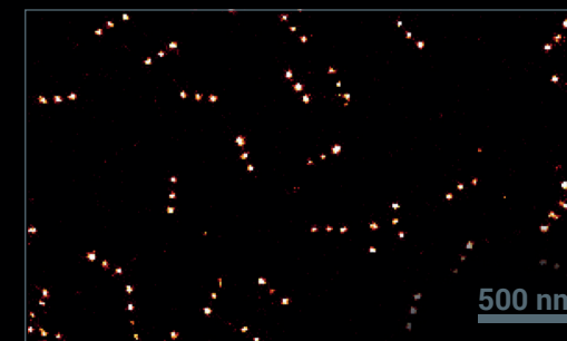
GATTA-PAINT 80R 3 spots with 80 nm distance and imaged with ATTO 655. Also available with fiducial markers for drift-correction.
